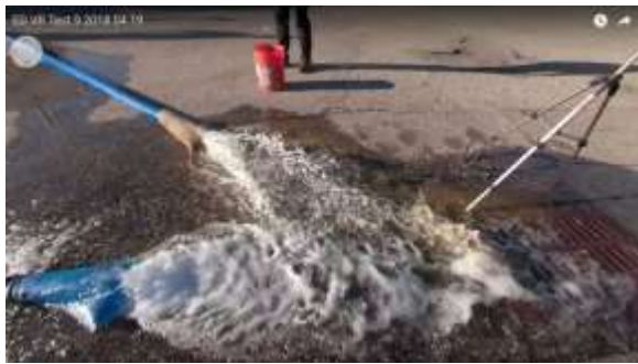
Image 19 - 500 gpm test of Device. Prior to the introduction of simulated trash
