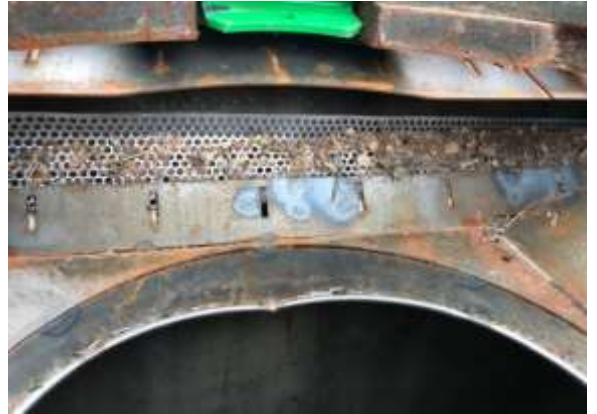
Image 7 - DIF with progressive overflow trash screen with Mundus Bag register visible in filter hanger
