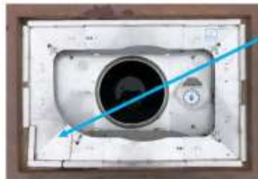
Figure 8 - Overhead view of hinged sample port on frame in a closed position
