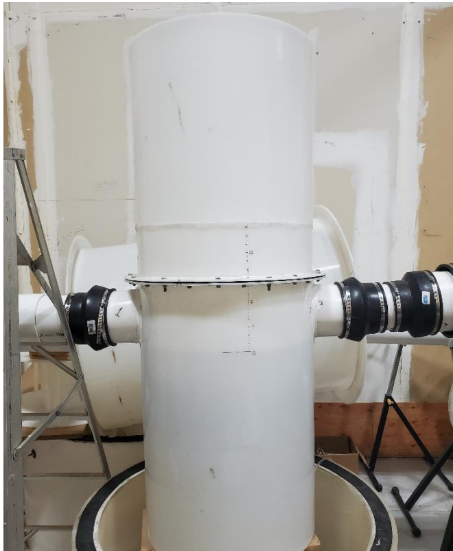
Figure 9. HydroDome TR (HDTs2-6) Installed in Hydroworks Laboratory (SIDE)
