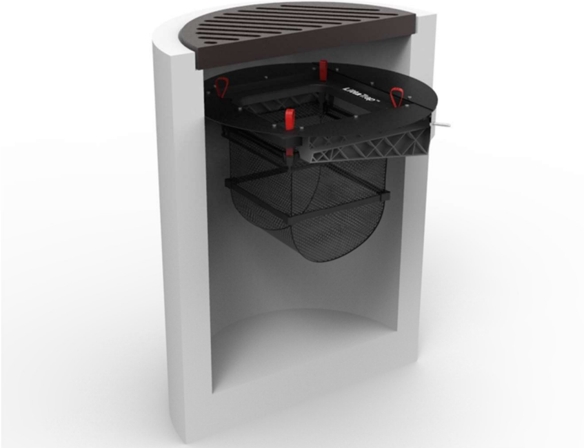
Figure 6 Illustration of the Enviropod® LittaTrap™ FC Manhole configuration.
