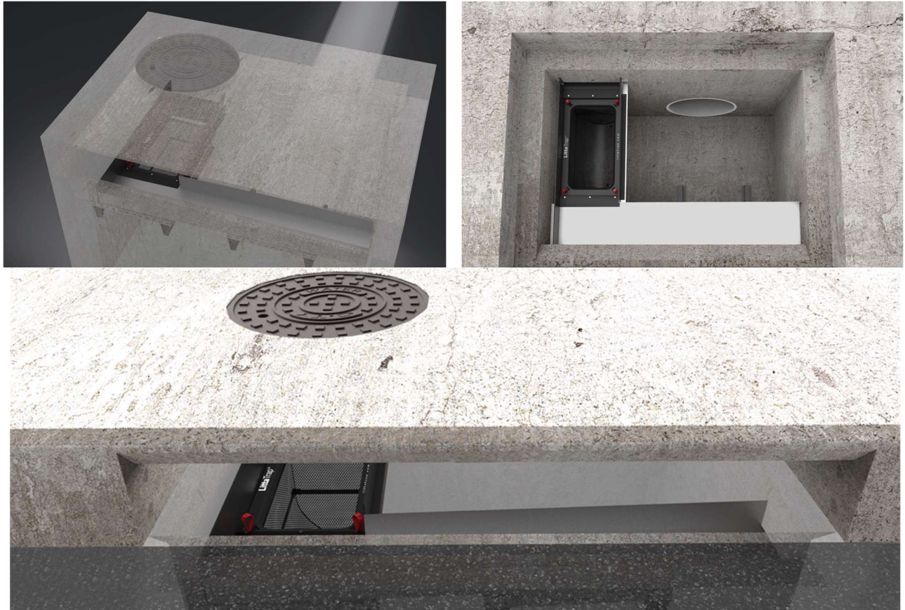
Figure 9 Enviropod® LittaTrap™ FC, Curb Inlet EMMA Configuration. Isometric view in catchbasin (top left) top view in catchbasin (top right) and street view looking into the curb inlet of a catchbasin (bottom). Note this configuration has one LittaTrap™ FC which receives flow via a feeder trough whereas the high-capacity configuration has multiple LittaTrap™ FC for the length of the inlet.
