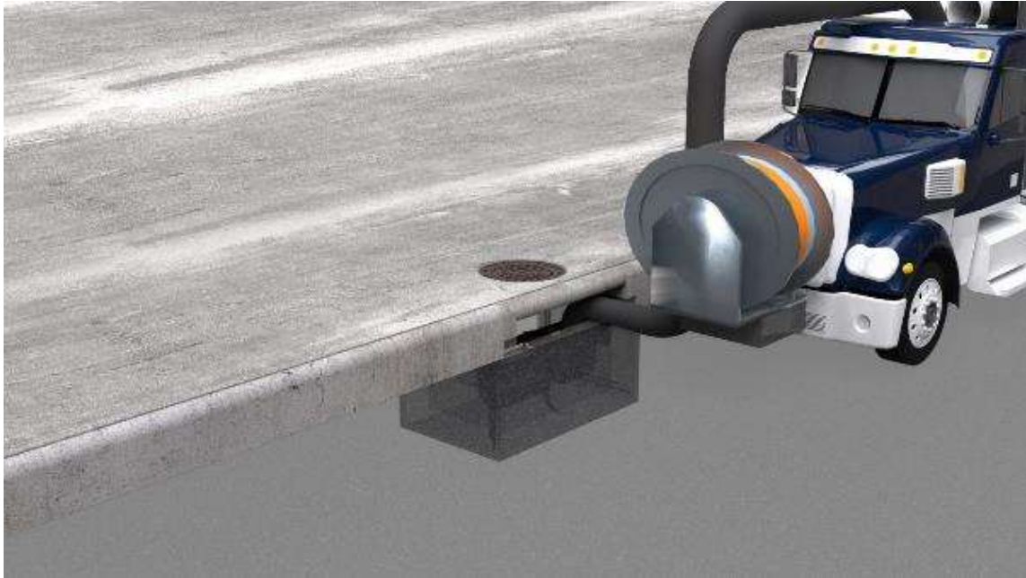
Figure 30 Illustration of an Enviropod® LittaTrap™ FC being maintained by a vactor hose through the curb opening.
