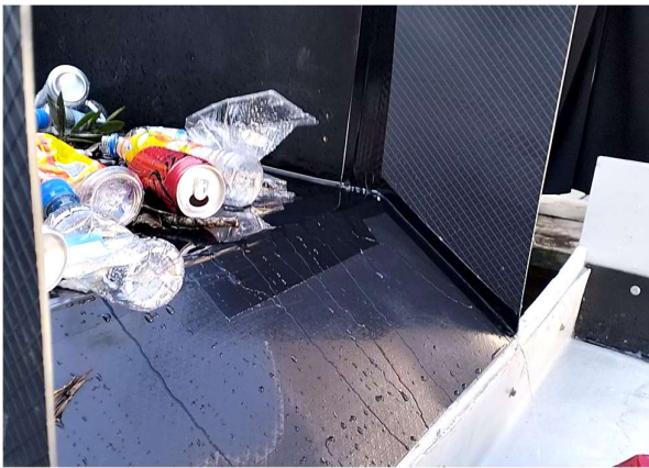
Figure 40 Photographs of testing ready to be carried out. Top: EMMA trough loaded with trash ready for testing. Note the 2 inch steel mesh screen extension to the back wall of the trough, which is the design modification. Bottom: Trash in the flume behind the steep catch basin inlet emulsion. Right: looking up the flume to the v-notch weir and the green water inlet.
