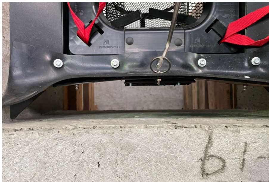
Figure 36: Enviropod® Littatrap™ FC with Vector Inspection in open position. The position and operation is the same for grated inlet catchbasins (Configuration 1), manhole catchbasins (Configuration 2) and combination inlet catchbasins (Configuration 3). Curb inlet configuration 4a and 4b do not require a vector port as they can be inspected via the manhole or inlet.
