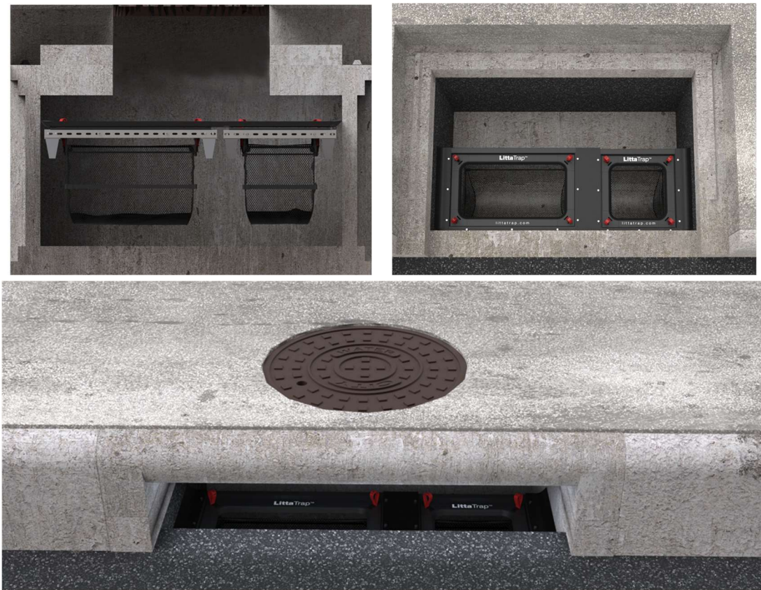
Figure 8 Enviropod® LittaTrap™ FC, Curb Inlet High-Capacity Configuration. Side view in catchbasin (top left) top view in catchbasin (top right) and street view looking into the curb inlet of a catchbasin (bottom). Note there are multiple LittaTrap™FC in this configuration, whereas the EMMA configuration only has one.
