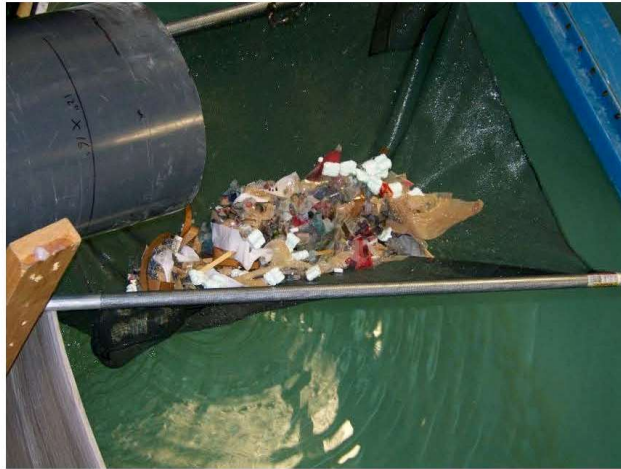
Figure 12: Escaped Solids – Control at 15 L/s
