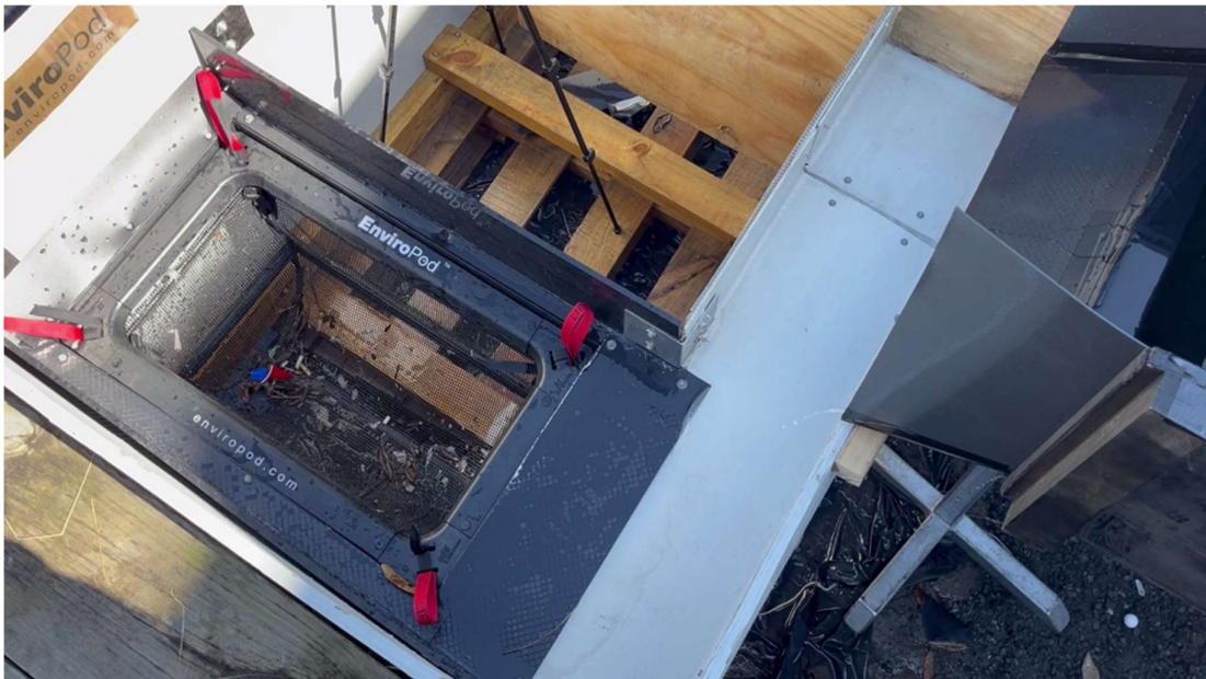
Figure 4 Plan view photograph of LittaTrap, EMMA trough and steep flume inlet as test set up.
