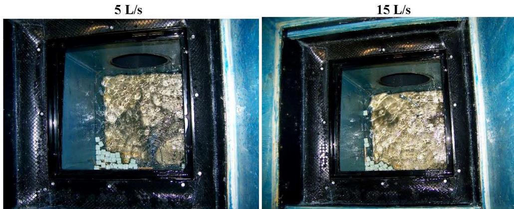
Figure 13: Retained Solids – Control at 5 and 15 L/S
